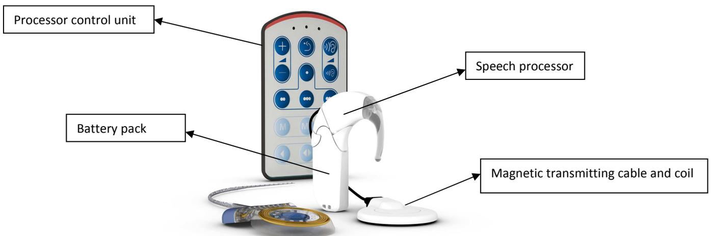
The external part of the ABI consists of a speech processor and battery pack that looks like a hearing aid. This fits behind the ear. The speech processor is attached via a cable to a magnetic transmitting coil that is positioned on the head over the magnetic, internal receiver stimulator package. The external parts of the implant can be removed at any time, for example when sleeping or swimming and bathing.
